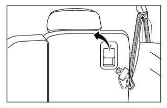
Lift the lever on the upper back corner of the seatback to move it to the desired position and then release it. Push and pull on the seatback to be sure it is locked in place.
